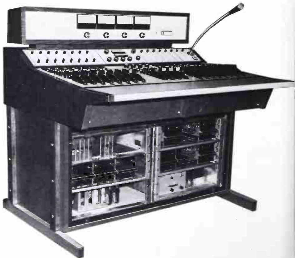
(Top) Custom audio console for WBEN-TV, Buffalo, has 11 inputs consisting of 11 pre-amps and one 6 X 18 high level input select panel. All channels have mixer modules (two with equalizers). Six have submaster modules. There is a custom built four-input telecine mixer. Monitor pushbuttons can look at three program channels. Unit has built in test oscillator.
